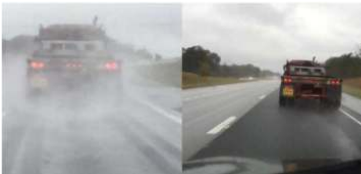
Fig. 5. Driver's view during rainy weather on a typical dense-graded pavement (left), and OGFC surface (right) [21]
